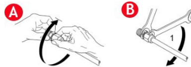
Wrap the Elbow fittings with new Teflon tape
