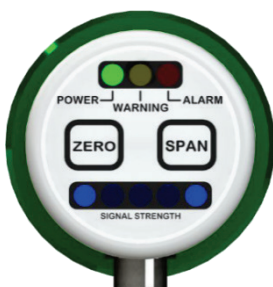
Figure 3-6: Automatic span calibration active after zero calibration
