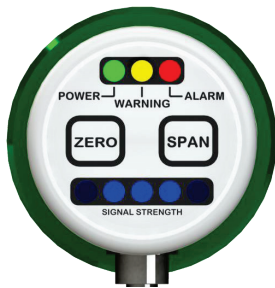
Figure 3-7: Automatic span calibration accepted
