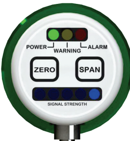
Figure 3-2: Strong signal, no obstructions to the light beam
