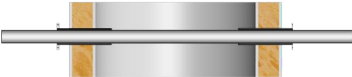
Figure 4-7, Opposite welding bracket alignment
