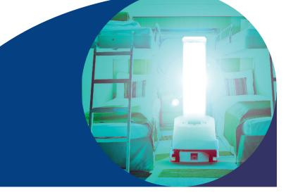
The UVD Robot emits UV-C light at 360 degrees, making it capable of decontaminating both air and surfaces from the floor to the ceiling. As the only device clinically proven to disinfect while on the move, it covers large areas in the shortest of times.
