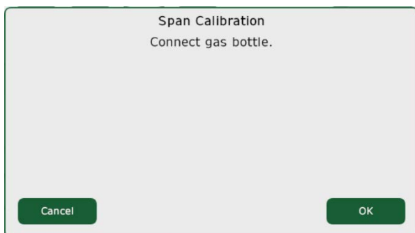
Figure 6-6, Span Calibration Connect Gas Bottle
