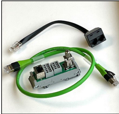
Figure 4-3, RTU Cable Kit
