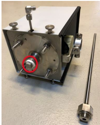
Figure 4-8, Removal of the Sealed Plug
